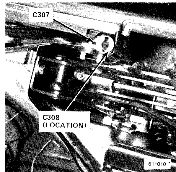
Figure 6 - RH Side of Soft Top Stowage Compartment
