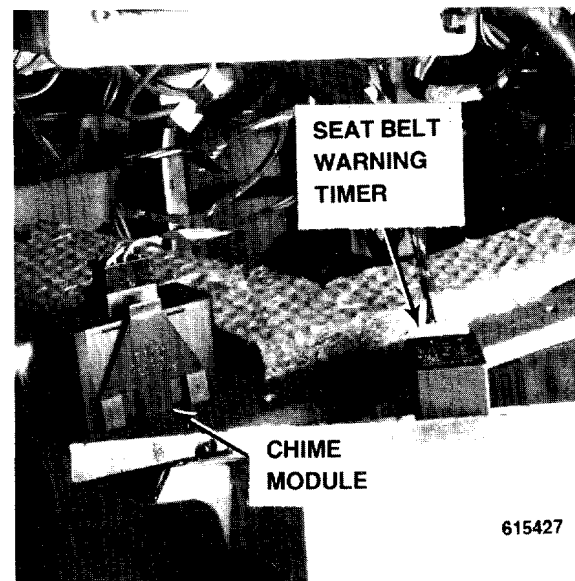
Figure 4 - Below LH Side of Dash, Left of Steering Column
